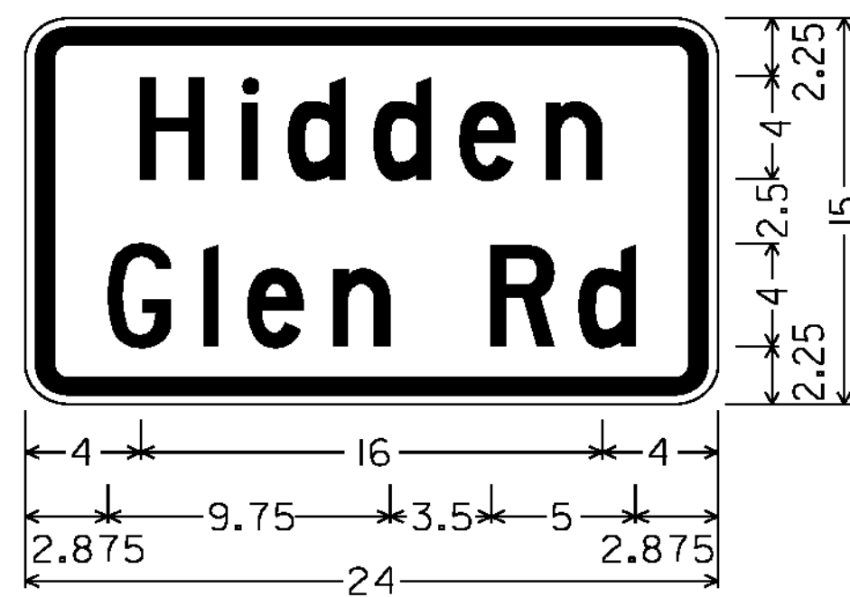
1.500" RADIUS, 0.625" BORDER, 0.375" INDENT, BLACK ON YELLOW; [Hidden] 4"C; [Glen Rd] 4"C W16-8P
