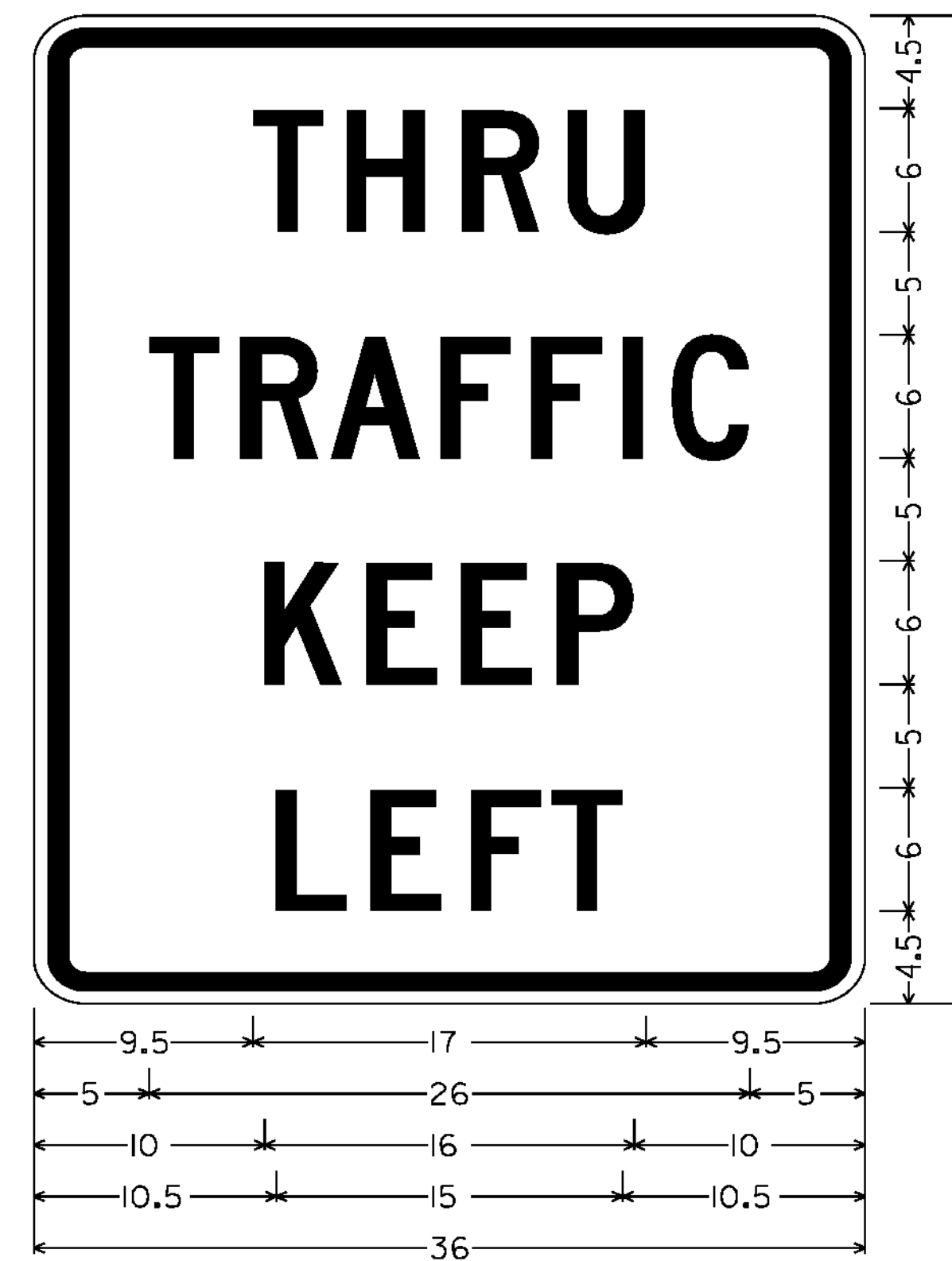
2.250" RADIUS, 0.875" BORDER, 0.625" INDENT, BLACK ON WHITE; [THRU] 2"C; [TRAFFIC] 2"C; [KEEP] 2"C; [LEFT] 2"C VR-118L
