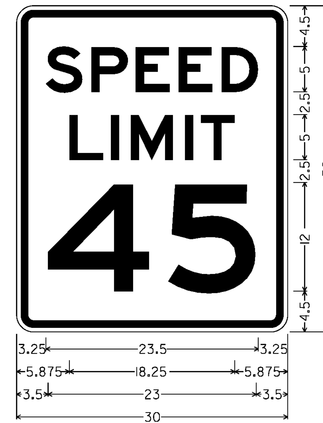
1.875" RADIUS, 0.750" BORDER, 0.500" INDENT, BLACK ON WHITE; [SPEED] 5"E; [LIMIT] 5"E; [45] 12"E R2-1
