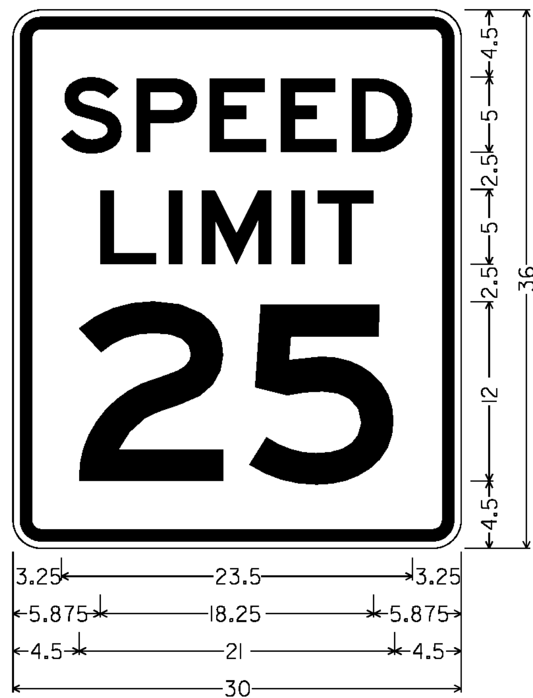
1.875" RADIUS, 0.750" BORDER, 0.500" INDENT, BLACK ON WHITE; [SPEED] 5"E; [LIMIT] 5"E; [25] 12"E R2-1
