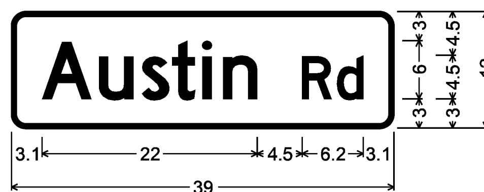
D3-1; 1.5" Radius, 0.5" Border, White on Green; [Austin] D 2K; [Rd] D 2K;
