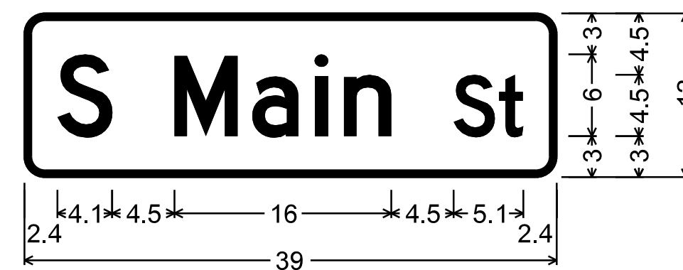
D3-1; 1.5" Radius, 0.5" Border, White on Green; [S Main] D 2K; [St] D 2K;
