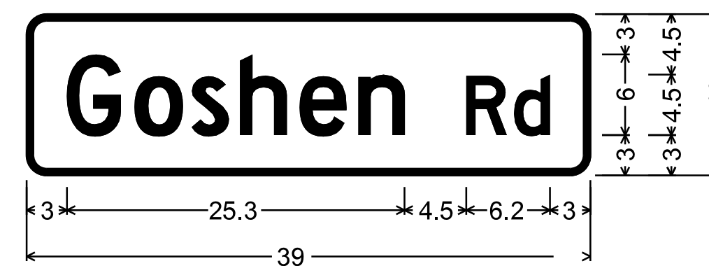
D3-1; 1.5" Radius, 0.5" Border, White on Green; [Goshen] D 2K; [Rd] D 2K;
