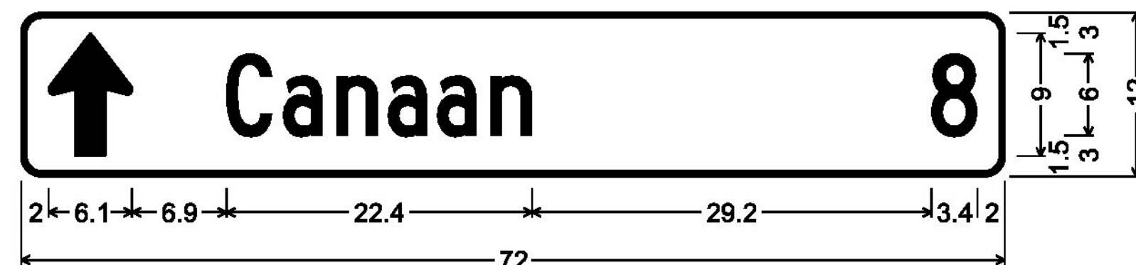
VD1-1A; 1.5" Radius, 0.4" Border, White on Green; Standard Arrow Custom 9.0" X 6.1" 90°; [Canaan] C 2K; [8] C 2K;
