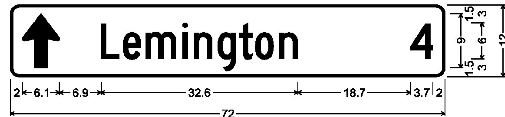
VD1-1A; 1.5" Radius, 0.4" Border, White on Green; Standard Arrow Custom 9.0" X 6.1" 90°; [Lemington] C 2K; [4] C 2K;
