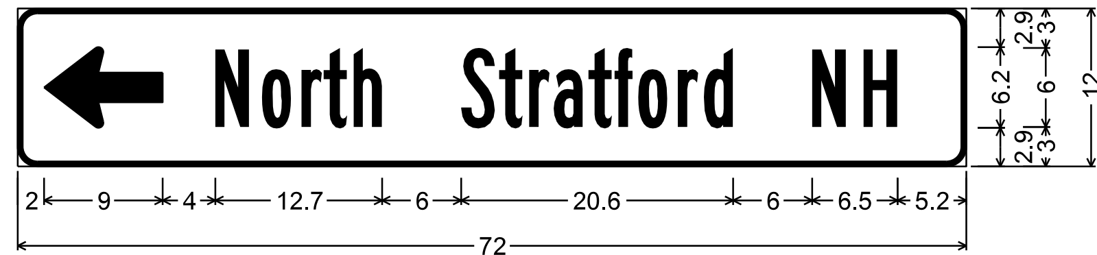
1.5" Radius, 0.4" Border, White on Green; Standard Arrow Custom 9.0" X 6.1" 180°; [North Stratford NH] B 2K;
