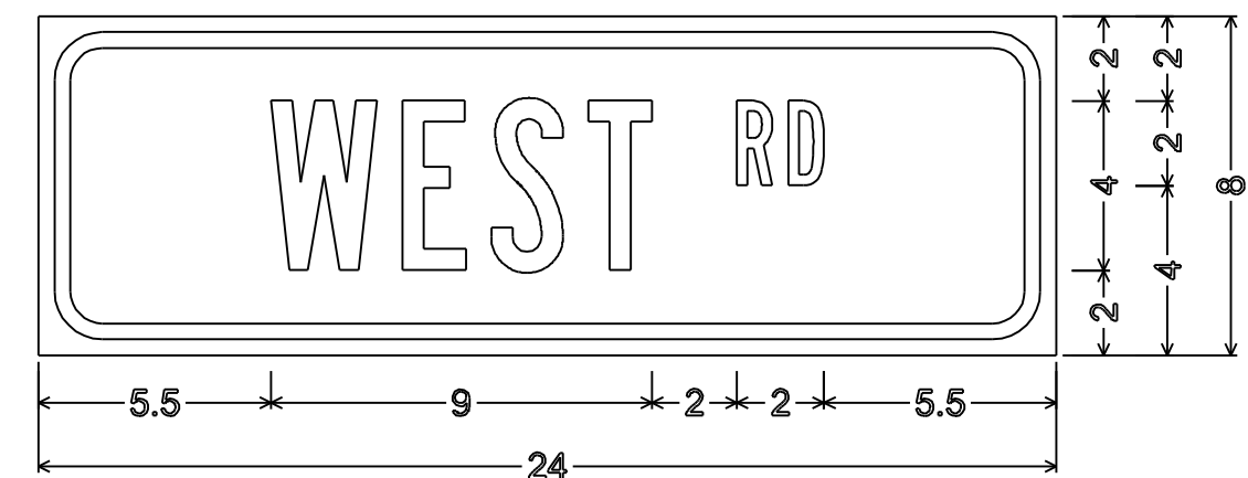
1.50" Radius, 0.38" Border, 0.38" Indent, Black on Yellow; "WEST RD" B; STA. 125+03.04, RT. STA. 133+21.44,LT.
