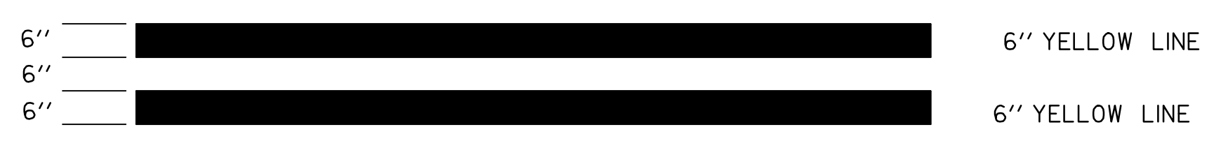
TYPICAL TWO-WAY RAMP CENTERLINE MARKING
