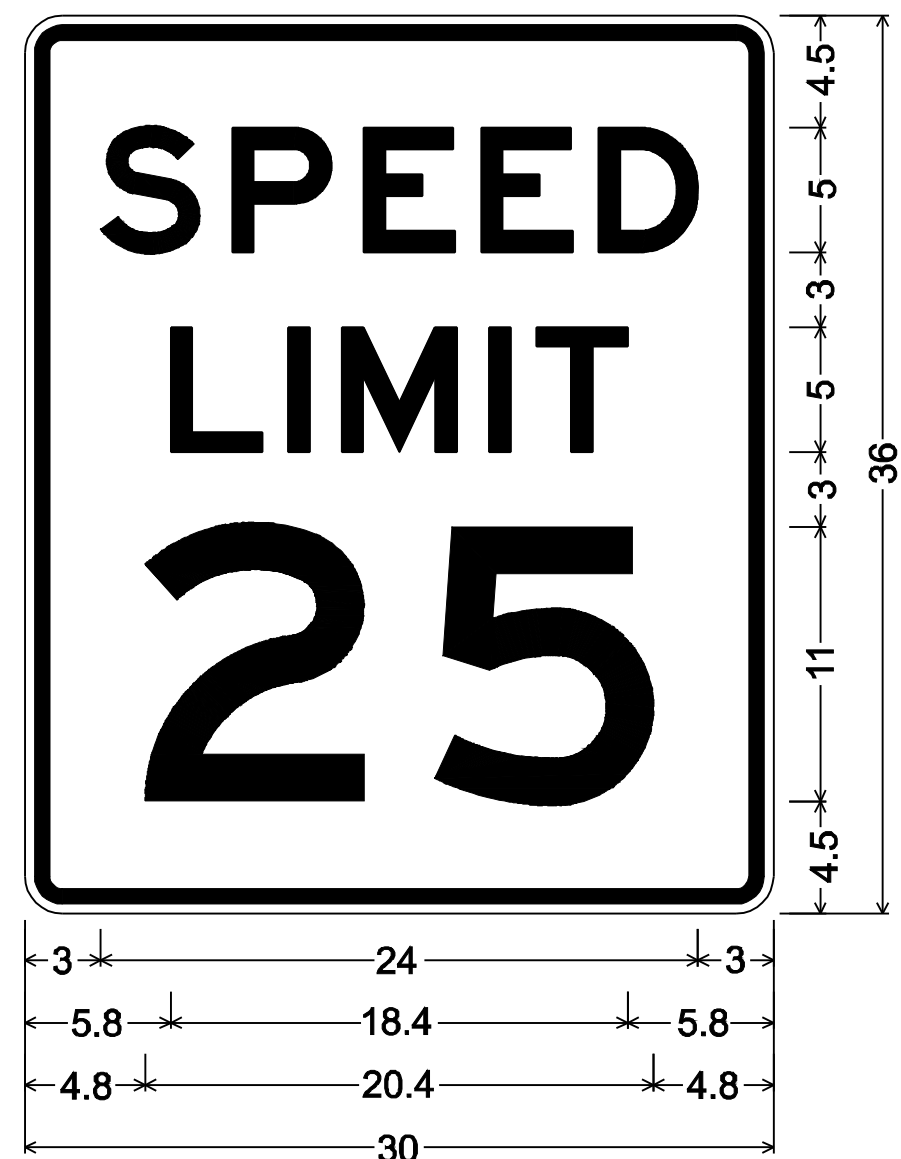
R2-1 STD; 1.5" Radius, 0.6" Border, 0.4" Indent, Black on White; "SPEED" E; "LIMIT" E; "25" E;
