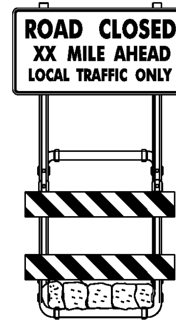
SIGN MOUNTING ON TYPE III BARRICADE (MODIFIED)
