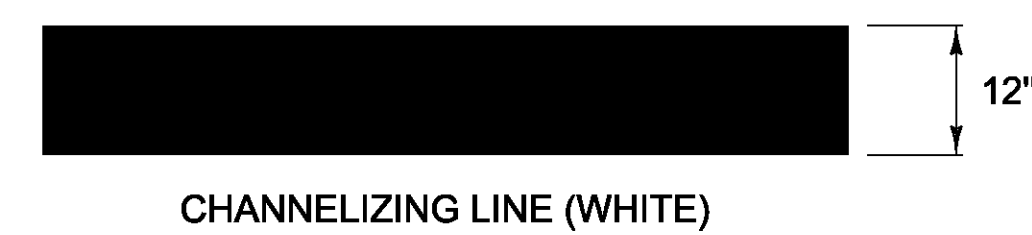
PAVEMENT MARKING LINE DETAILS NOT TO SCALE
