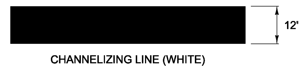
PAVEMENT MARKING LINE DETAILS NOT TO SCALE
