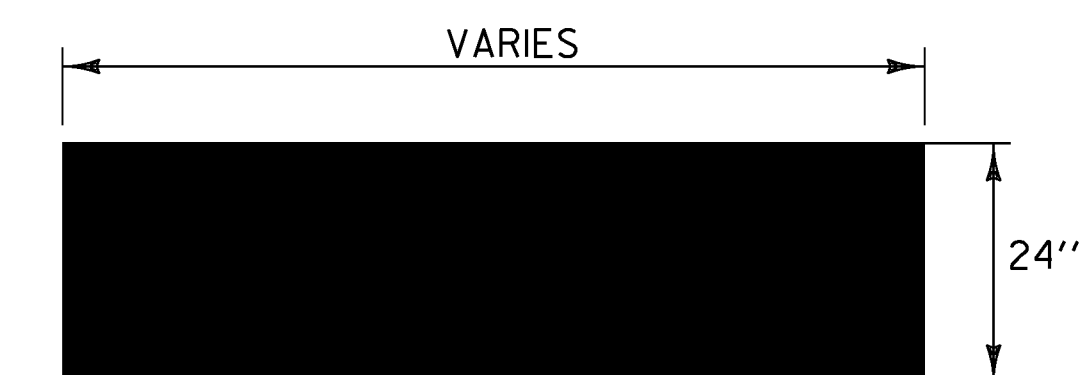
STOP BAR DETAIL NOT TO SCALE
