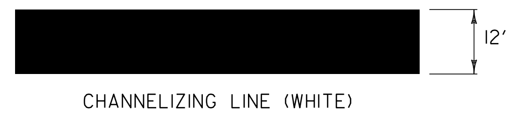
PAVEMENT MARKING LINE DETAILS NOT TO SCALE
