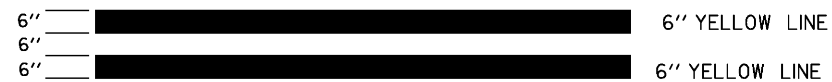
TYPICAL TWO-WAY RAMP CENTERLINE MARKING
