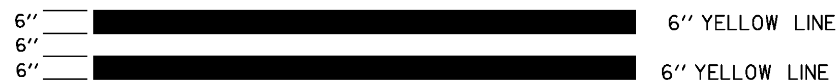
TYPICAL TWO-WAY RAMP CENTERLINE MARKING
