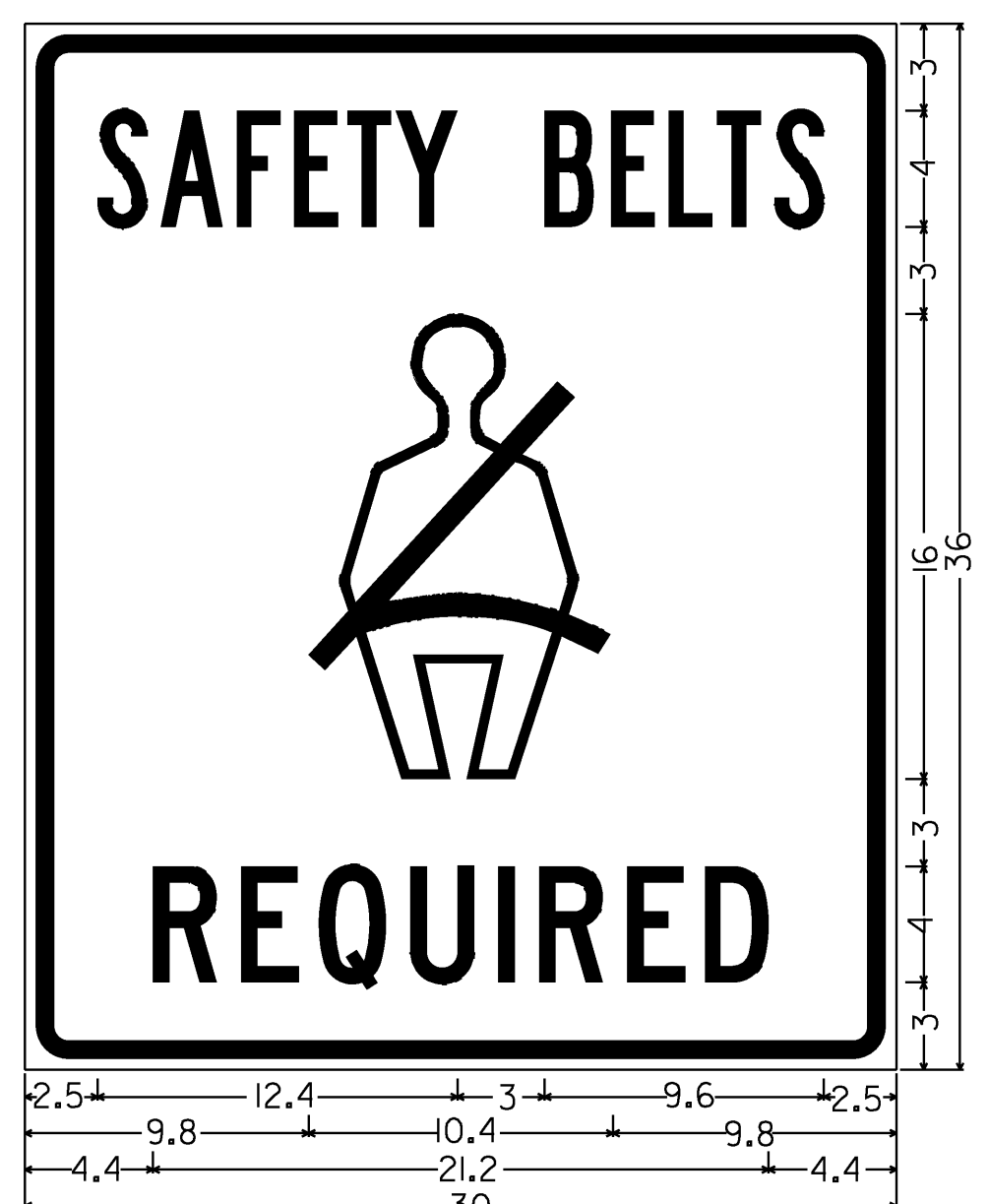
1.5" Radius, 0.6" Border, 0.4" Indent, Black on White; *SAFETY BELTS" B specified length; Symbol RG015; *REQUIRED" C;
