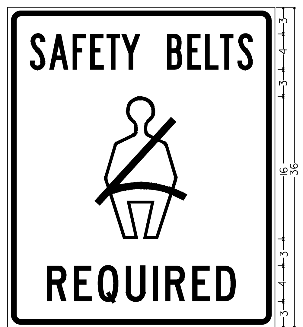
1.5" Radius, 0.6" Border, 0.4" Indent, Black on White; *SAFETY BELTS" B specified length; Symbol RG015; *REQUIRED" C;
