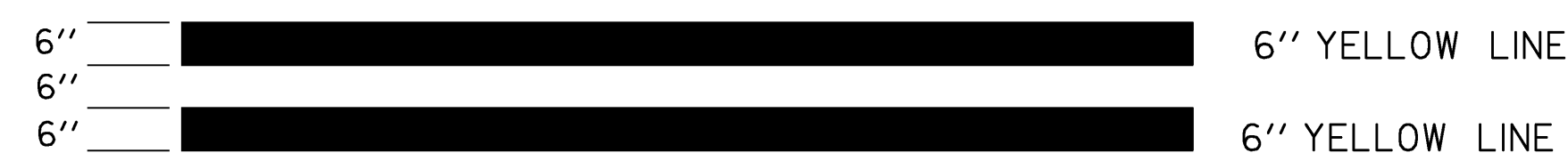
TYPICAL TWO-WAY RAMP CENTERLINE MARKING
