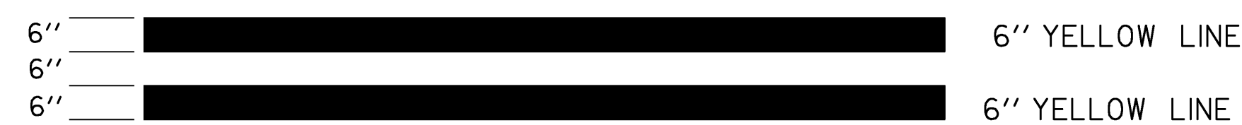
TYPICAL TWO-WAY RAMP CENTERLINE MARKING
