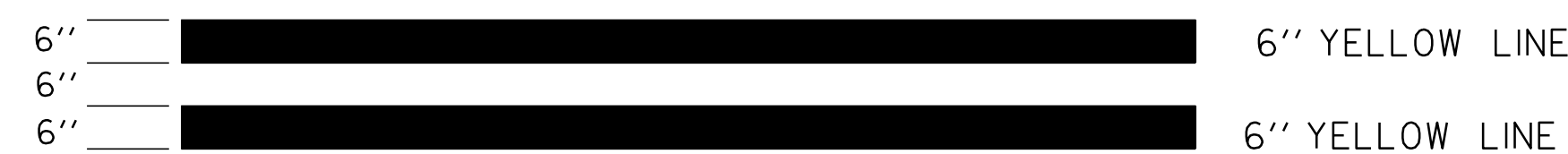
TYPICAL TWO-WAY RAMP CENTERLINE MARKING
