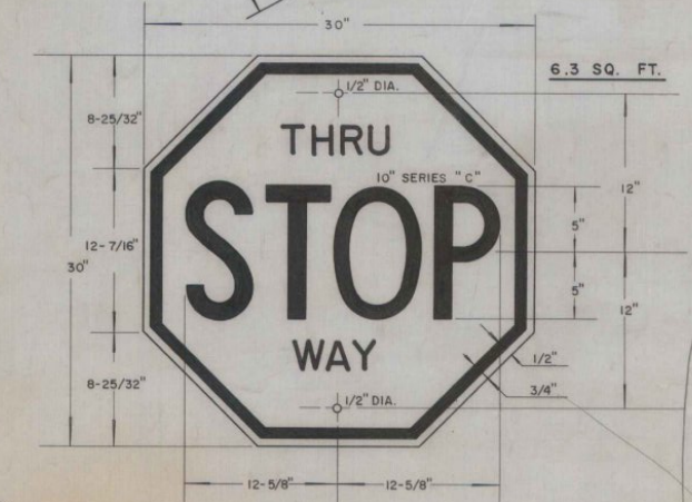
(C) REFLECTORIZED SILVER TEXT ON A REFLECTORIZED RED BACKGROUND.
