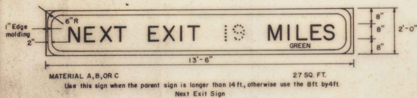
NEXT EXIT SIGN:
