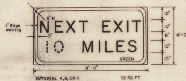
NEXT EXIT SIGN:
