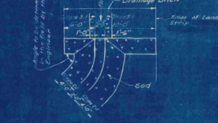
DETAIL OF TRANSITION BETWEEN DRAINAGE DITCH AND SOD GUTTER AT STA. 11+30
