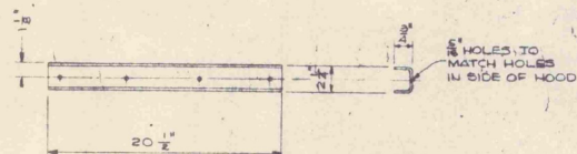
① SIDE FILTER GUIDE 16 GA. GALV. 2 REQ.
