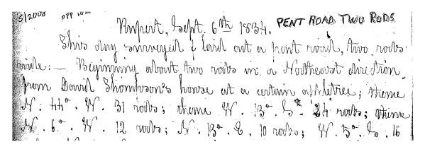
The above reads as: "Rupert, Sept. 6<sup>th</sup> 1834. This day surveyed & laid out a pent road, two rods wide: \_\_\_ Beginning about two rods in a Northeast direction from David Thompson's house at a certain appletree; thence N. 44° W. 31 rods; thence W. 13° S. 24 rods; thence N. 6° W. 12 rods; N. 13° E. 10 rods; W. 5° S. 16 ..."
