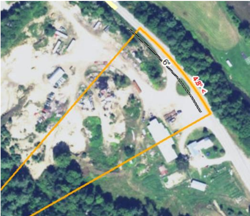
Figure 7 : Example Curve Comparison between VTrans legacy data and latest calculated values using Curve and Grade Tools for ArcGIS by Works Consulting. The orange wedge represents the latest calculated B-curve – whereas the black line is shown offset from the centerline on the inside of the curve to see how it starts and ends at different locations compared to the orange wedge.
